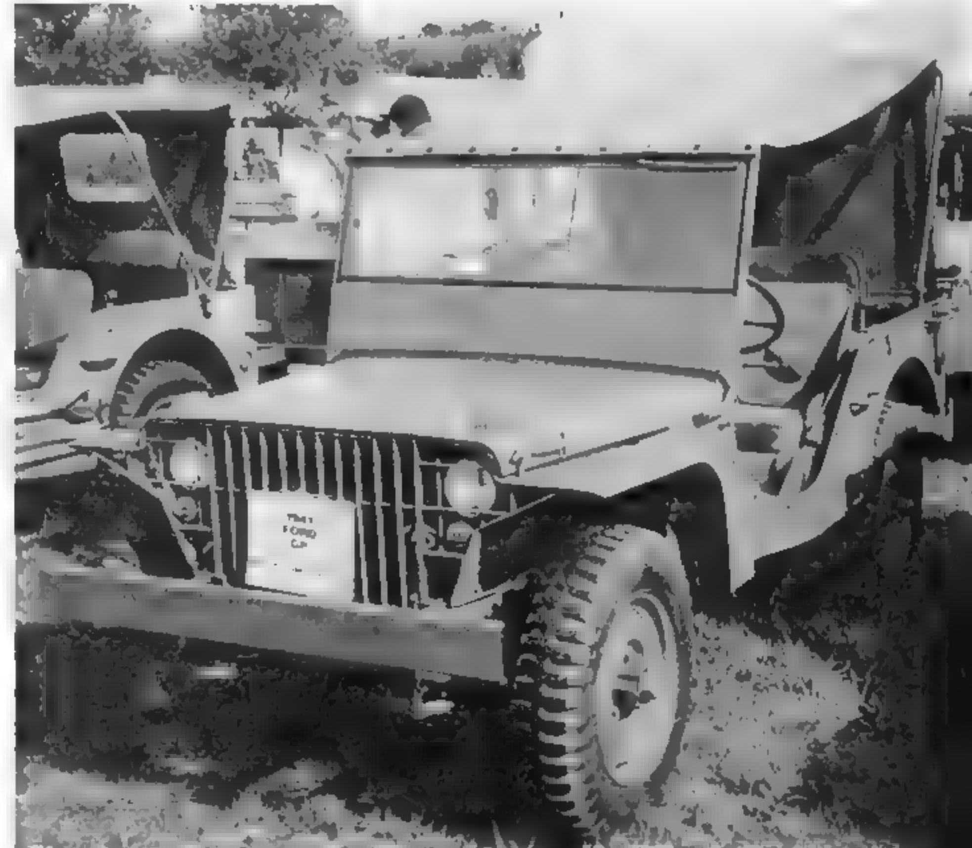
During the field evaluation period, the Army ordered 1,500 vehicles of the improved GP model from Ford. These vehicles had fabricated "slat" grilles.
